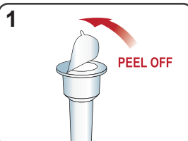
1. Peel off aluminum foil seal from the top of the extraction vial containing the extraction buffer.
